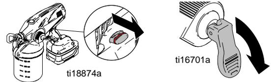
4. Engage trigger lock. Put prime/spray valve UP to release pressure and rotate spray tip back to SPRAY position.
