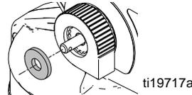
6. Install valve handle onto stem.
