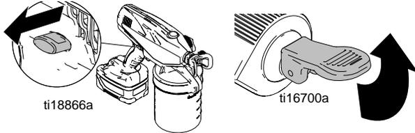
2. Install material cup liner, fill with material, and thread onto sprayer.
