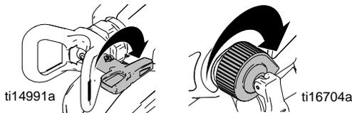
3. Aim sprayer at waste area, disengage trigger lock, and put prime/spray valve DOWN to spray position. Pull trigger to clear clog.
