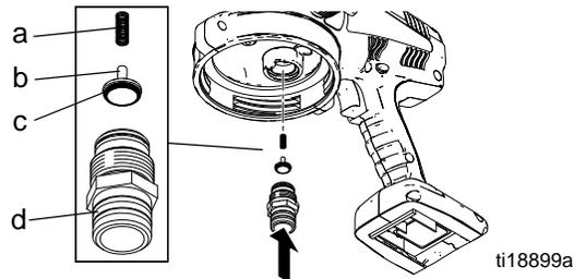
2. Hold inlet in place and turn sprayer upside-down. Remove inlet valve fitting and visually check to see that inlet valve has seated correctly.
