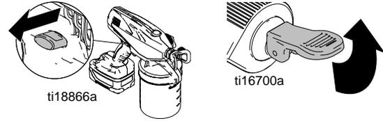
**NOTE:** Air vent holes or the air vent valve (as your model is equipped) allow air to flow into the material cup while spraying to prevent loss of fluid flow.
