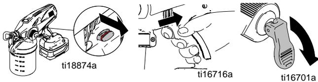
4. Reverse spray tip to UNCLOG position, pull trigger and release.
