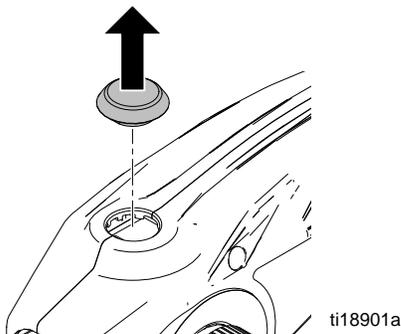
4. Use tool (supplied) to loosen and remove outlet valve fitting. Make sure old o-ring, seat, outlet valve fitting, and spring are out of pump outlet cavity.
