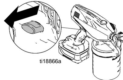
2. Put prime/spray valve UP to release pressure.
