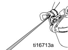
5. Engage trigger lock and put prime/spray valve UP to release pressure.
