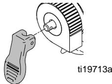
7. Insert pin into valve handle. Use pliers to press pin into hole.
