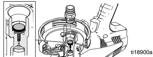
3. Replace inlet fitting and use wrench or socket to tighten to 10 ft-lb (14 N•m).
