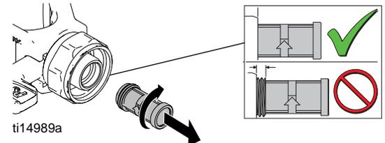
**NOTE:** Spray tip filter assembly is reverse-threaded: **Turn left** (or counter-clockwise) to install. **Turn right** (or clockwise) to remove.
