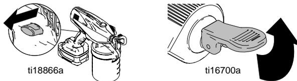
2. Reverse spray tip to UNCLOG position. Turn pressure control knob to maximum pressure setting.
