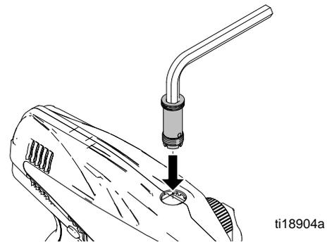
2. Press outlet valve fitting access plug into place.
