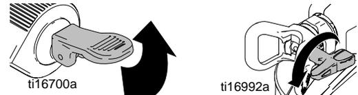
5. Disengage trigger lock, put prime/spray valve DOWN to spray position, and resume spraying.
