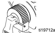
**NOTE:** If pin does not assemble, repeat steps 3 - 6 to ensure pressure control is fully engaged with retainer.
