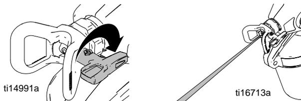
5. Put prime/spray valve UP to release pressure. Then rotate spray tip back to spray position.
