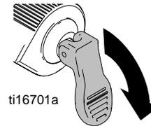
4. Reverse Spray Tip to UNCLOG position and trigger sprayer into a waste area for 10 seconds.
