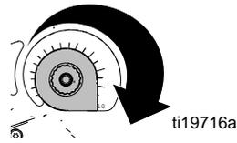
**NOTE:** You may have to rotate pressure control knob slightly counter-clockwise to fully engage pressure control knob with retainer.
