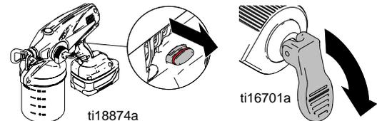
6. If spray tip is still clogged, you may have to repeat steps 1 - 5 and rotate the spray tip from SPRAY to UNCLOG several times. Repeat step 1 to release pressure, remove and clean spray tip filter, or replace with new spray tip/guard assembly.
