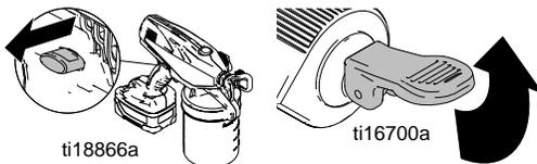
2. Remove material cup, flexible suction tube, and battery.
