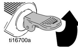
3. Put prime/spray valve DOWN to spray position.
