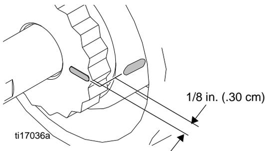
4. Position pressure control knob in fully clockwise position and press firmly onto retainer.
