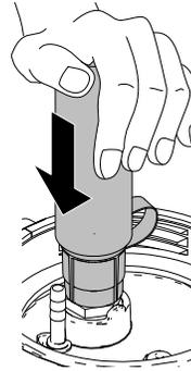
2. Clean air vent holes or the air vent valve, depending on model. See **Shutdown and Cleaning**, page 15. Remove air vent valve, clean, and reinstall.
