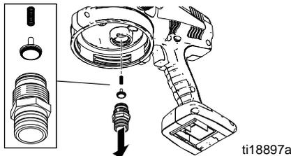
**NOTE:** Make sure the spring also comes out. Use needle-nose pliers to remove if needed. Inlet cavity should be completely empty (as shown below).
