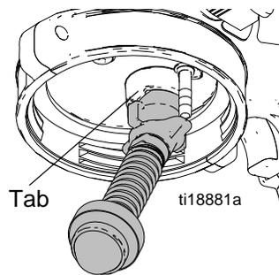
**NOTE:** If the sprayer is angled or tilted too far, the flexible suction tube will lose contact with the material and the sprayer will stop spraying.
