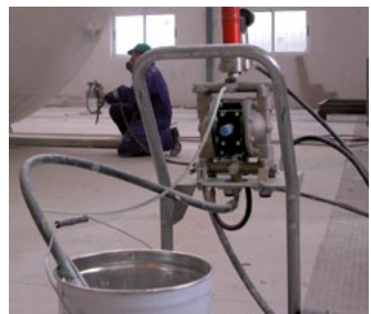
Absorption probe (suction)
