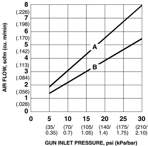
**Atomizing Air Pressure; Compliant Air Cap 241563**
