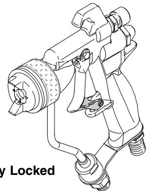
Gun Trigger Safety Locked
