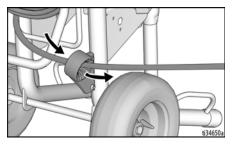
Lift and turn pivot lock 90° to unlock Hose Reel. Pull on Hose to remove it from Hose Reel.
