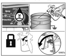
Turn Pressure Control Knob to OFF and turn ON/OFF switch to OFF position. Disconnect power to sprayer.
