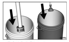
To flush Drain Tube and pump turn Prime/Spray Valve down to PRIME position.
