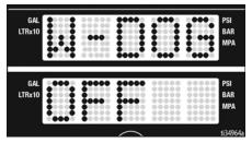
Short press **DISPLAY** button to move to WatchDog sensitivity menu. Press and hold **DISPLAY** button and Watchdog can be set to low, medium, or high sensitivity. Release **DISPLAY** button when desired sensitivity setting is displayed. Default is medium.
