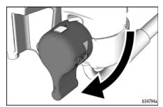
Hold the Spray Gun firmly to a grounded pail. Point Spray Gun into pail. Disengage the Trigger Lock and trigger the Spray Gun to relieve pressure.
