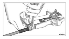
When unpacking sprayer for the first time remove packaging materials from inlet strainer. After long term storage check inlet strainer for clogs and debris.
