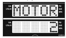
Short press DISPLAY button. LAST CODE scrolls by and last code is displayed; e.g. CODE 06 MOTOR THERMAL PROTECTION ENABLED (see Repair manual).
