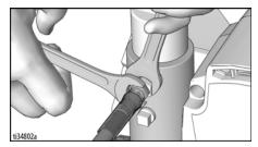
Connect Spray Gun to other end of Hose. Use wrenches to tighten securely.
