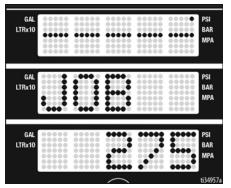
Press and hold the **DISPLAY** button to reset to zero.
