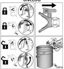
**NOTE:** If Spray Tip is difficult to rotate when turning to the UNCLOG position perform, **Pressure Relief Procedure**, page 19, then turn Prime/Spray Valve horizontal to SPRAY position and repeat step 1.
