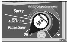
Put Drain Tube into a waste pail and turn Prime/Spray Valve down to PRIME position to relieve pressure.
