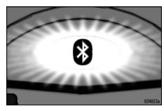
Blinking red LED total count equals the error code (for example: two blinks equals CODE 02).
