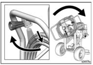
**NOTE:** QuikReel can be locked into two positions: Usage (A) and Storage (B).
