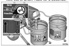
7. Turn Pressure Control Knob to OFF setting (all the way counterclockwise).
