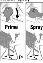
The Prime/Spray Valve directs the fluid to either the Drain Tube or the Hose and Spray Gun. It is used to prime the sprayer, which means to evacuate the air out of the pump, Hose, and Spray Gun.
