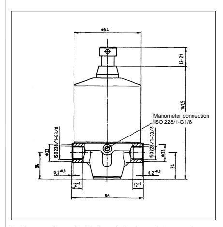
Build-up position Vertical, regulating key points upwards
