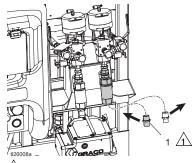
$\triangle$  Apply thread sealant (5) to threads.
