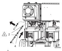
$\triangle$  Apply thread sealant (5) to threads.
