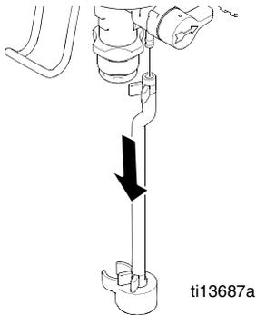
4. Remove hopper lid. Insert hopper into pump.
