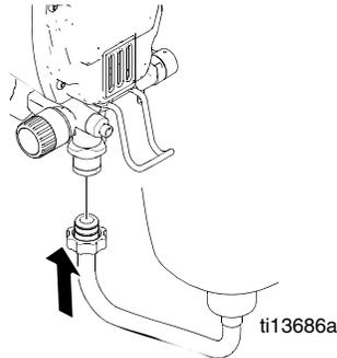
5. Tighten jam nut until hopper does not move.
