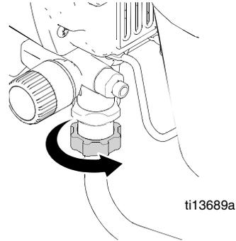
6. Replace drain tube with longer tube and place into hopper. Push drain tube fully onto barbs with hose clamps in place.
