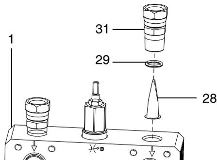
2. Pull “V” screen (28) and retainer o-ring (29) straight up and out with a needle nose pliers.
