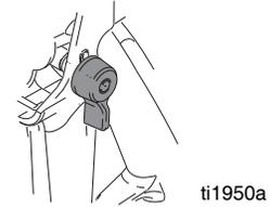
5. Hold the metal part of the gun firmly to a grounded metal pail with a lid to avoid splashing. Trigger the gun until mixed coating material is evident and purge solvent is gone.
