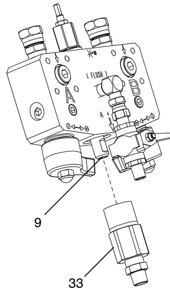
2. Clean any build-up on, around, or inside the tube (9).
