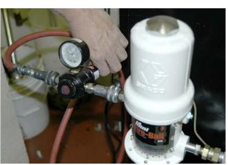
2. Set air regulator pressure to zero psi and/or turn off main air supply.
