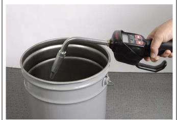
3. Trigger the dispense valve into a waste fluid container to relieve fluid pressure.
