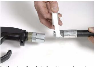
6. Wrap hose thread with thread tape as shown above.
