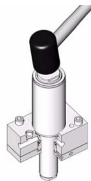
Seat Cylinder in Bore
