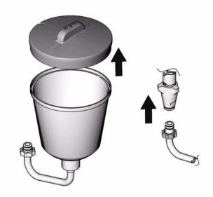
3. Remove hopper lid. Insert hopper tube into pump.
