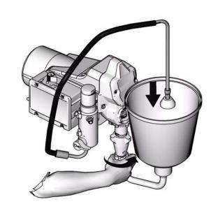
4. Hand-tighten jam nut. Place drain tube into hopper.
