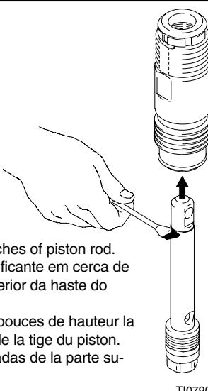
Grease top two inches of piston rod.
