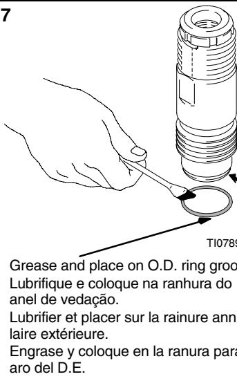
Grease and place on O.D. ring groove
