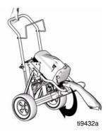
Slide suction tube under hook (b) in back of sprayer cart.
