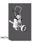
For compact, shelf storage, loosen, but do not remove, wingnuts (c) and fold handle down as shown.
