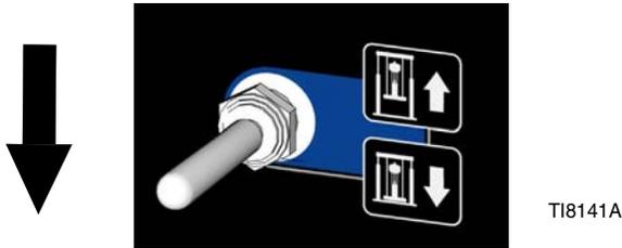
3. When the ram reaches the full down position, place the ram UP/DOWN lever in the center position (off).
