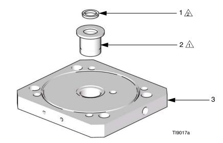
$\underline{\land}$  Press fit bushing with flange bottomed against counterbore step.
