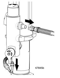
5. Using a wrench, loosen filter housing fitting (110) and remove housing from pump.
