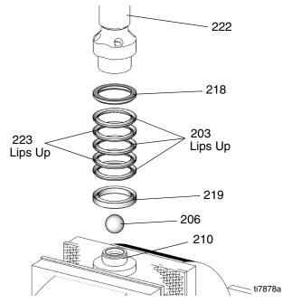
5. Clean all parts with a compatible solvent and inspect them for wear or damage. Replace any worn parts.
