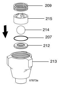
Place intake valve (213) assembly in vice. Install cylinder (205) assembly to intake valve. Torque to 350 ft-lb (475 N•m).
