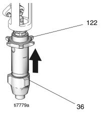
Hand tighten jam nut (122). Then tighten securely 1/8 to 1/4 turn with hammer or torque to 330 ft-lb (447.4 N•m).
