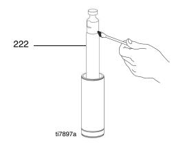
6. Grease o-ring (207) and place on sleeve. Slide one o-ring (207) inside cylinder (205). Slide sleeve/piston rod assembly (222) into bottom of cylinder.
