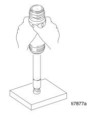
Component Rupture Hazard. Do not clean or wipe piston valve threads. Cleaning the piston valve threads could destroy the special sealing patch and cause the piston valve to come loose during operation, causing pump bursting and possible serious bodily injury.
