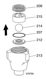
3. Select proper ball travel for material sprayed. Reassemble as shown.
