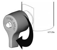
If you suspect that the spray tip or hose is completely clogged, or that pressure has not been fully relieved after following the steps above, VERY SLOWLY, loosen tip guard retaining nut or hose end coupling to relieve pressure gradually, then loosen completely. Then clean tip and hose.
