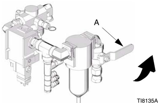
3. Disengage trigger lock.
