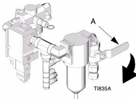
2. Place the ram UP/DOWN lever in the UP position.
