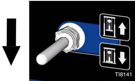
3. When the ram reaches the full down position, place the ram UP/DOWN lever in the center position (off).
