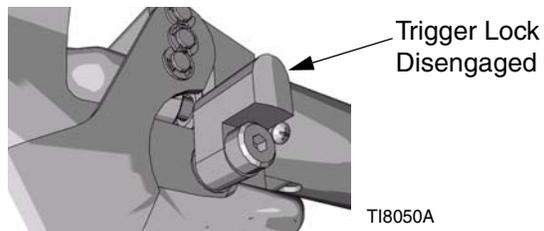
4. Hold a metal part of the gun firmly to a grounded metal pail. Trigger the gun to relieve pressure.
