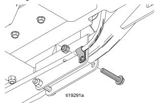
3. NOTE: The orientation of the new clamp must allow room for the recoil tube.
