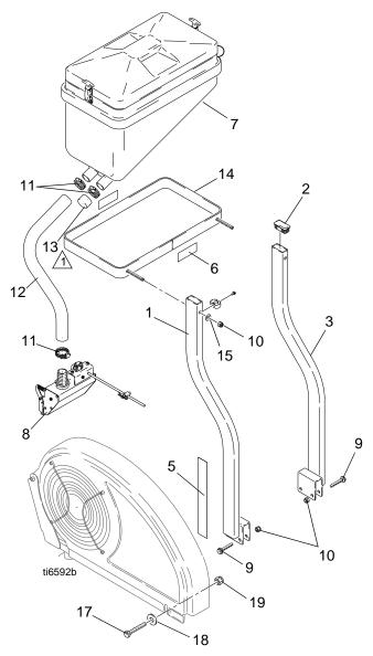
Remove cap (13) and install second hose (12) and clamp (11) for 12-inch bead dispenser
