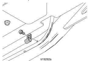
2. Install new clamp to secure recoil tube to new mounting bracket.
