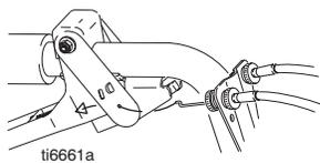
5 Insert gun cable in gun selector plate
