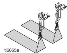
8 Adjust cable and gun trigger so both guns trigger at the same time.
