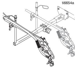
1 Install extension clamp (10) and extension support bracket (12)
