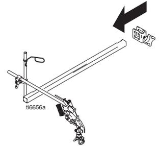
b Slide extension clamp onto existing gun arm support bracket
