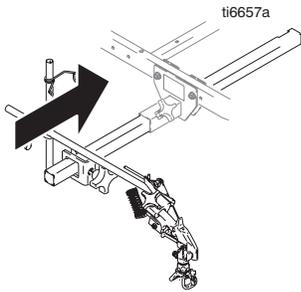
c Install existing gun support bracket.
