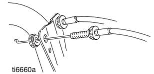
4 Insert gun cable through cable bracket. Install and tighten knurled nut.
