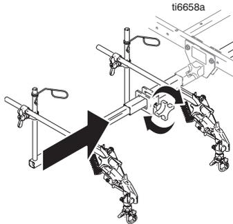
2 Install extension support bracket (12). Tighten extension clamp (10).
