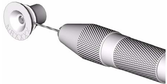
FIG. 1. Cleaning Component A (ISO) Ports
