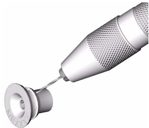
FIG. 2. Cleaning Component B (Resin) Ports
