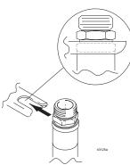
3. Align dots located on hose fitting, making sure they are facing each other at all times to ensure the hose does not twist during reinstallation.
