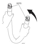
Slide hose onto plate as shown below, making sure plate slides into slot between hex fitting on end of hose.
