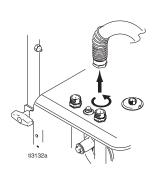
8. Rotate plate. Slide hose off by pushing outward on hose fittings.
