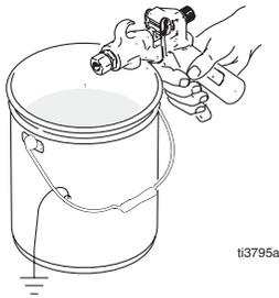
1. **Pump:** connect a ground wire and clamp to a true earth ground as shown in pump manual.
