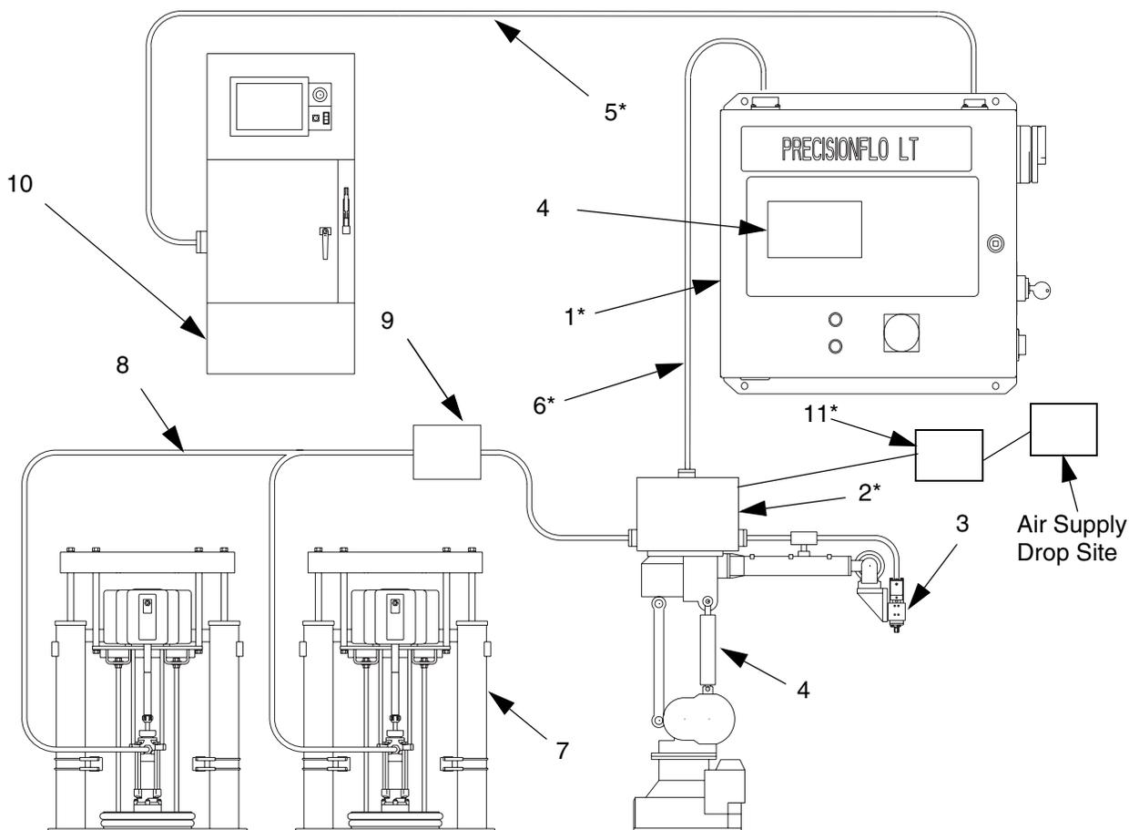
**Note:** For proper operation of filter assembly, filter orientation must be such that the bowls are orientated so the bowls are always perpendicular to the ground (i.e. do not attach to robotic arms, as the filters may not remain in the proper orientation.)
