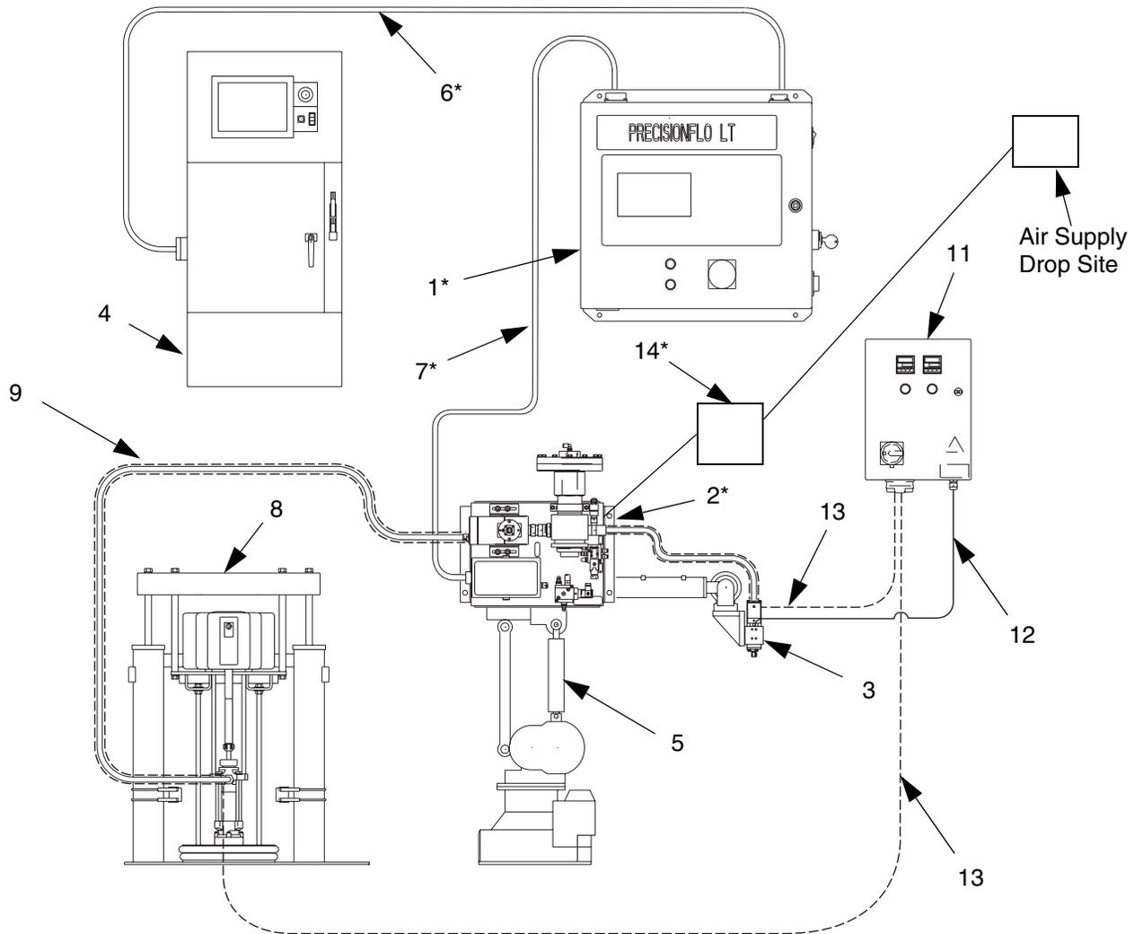
**Note:** For proper operation of filter assembly, filter orientation must be such that the bowls are orientated so the bowls are always perpendicular to the ground (i.e. do not attach to robotic arms, as the filters may not remain in the proper orientation.)
