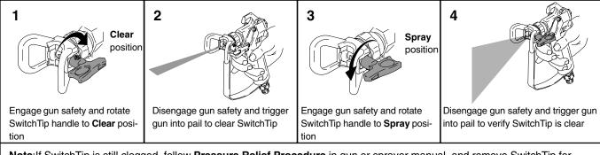
Note: If SwitchTip is still clogged, follow Pressure Relief Procedure in gun or sprayer manual, and remove SwitchTip for cleaning.
