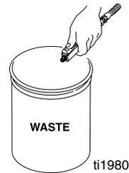
5. Turn ON sprayer power switch. Align arrow on sprayer and pail symbol on pressure control knob.
