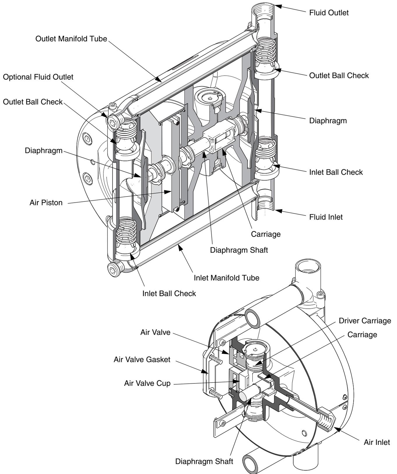
**FIG. 5. Cutaway Views of Pump and Air Valve**
