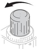
3. Open the pump's bleed-type master air valve (B).
