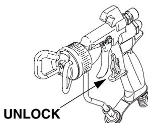
4. Trigger the gun into a grounded metal waste container to relieve the fluid pressure.
