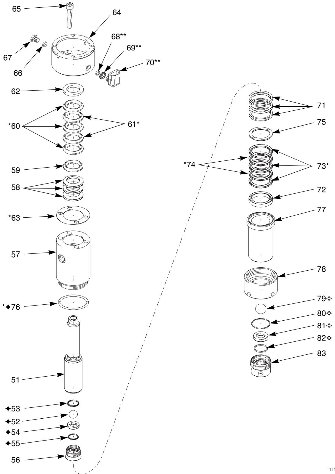
**Part No. 245351 020 Displacement Pump, Series A****Part No. 245352 050 Displacement Pump, Series A****Part No. 245353 035 Displacement Pump, Series A**
