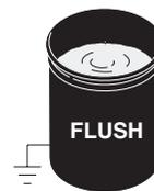
4. Hold a metal part of the gun firmly to the side of a grounded metal pail.
