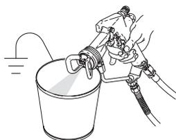
2. Remove the spray tip from the gun. See the gun manual.
