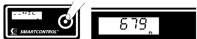
**Note:** Displays the linear line length applied since the last reset. See Reset screen, step 9.
