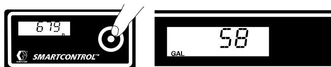
**Note:** Displays material sprayed (gallons or liters x 10) since the last reset.
