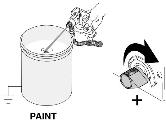
11. Hold gun against paint pail. Take trigger safety **OFF**. Trigger gun until flushing fluid appears.
