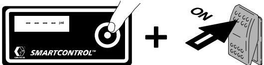
2. Simultaneously press DTS button and set pump on/off switch on.
