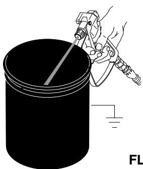
10. Trigger gun again into flushing fluid pail until paint appears. Assemble tip and guard, page 8.
