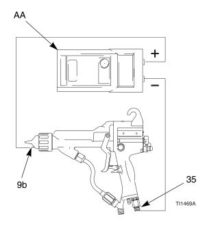
Fig. 5. Test Gun Resistance
