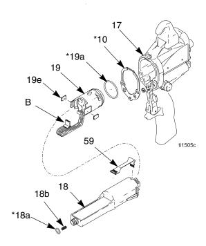
Fig. 18. Power Supply and Turbine Alternator
