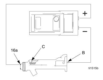
Fig. 7. Test Barrel Resistance
