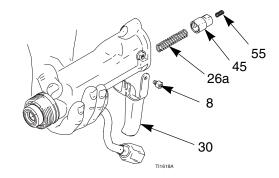
Fig. 13. Spring Cap and Springs
