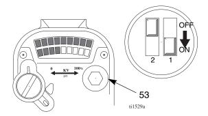
Fig. 4. Low Voltage Adjustment Switches
