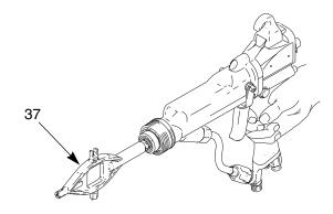
Fig. 9. Seat Housing Replacement
