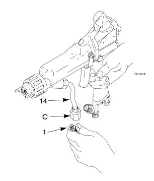
Fig. 12. Fluid Filter Removal
