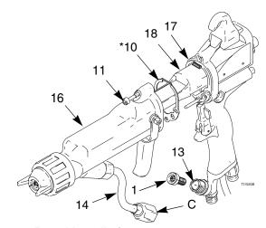
Fig. 17. Barrel Installation
