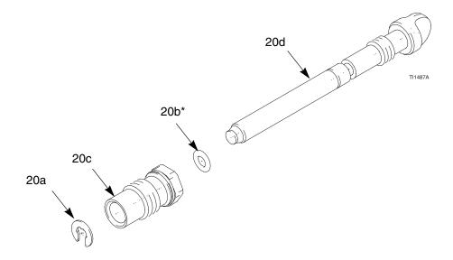
Fig. 19. Atomizing Air Adjustment Valve
