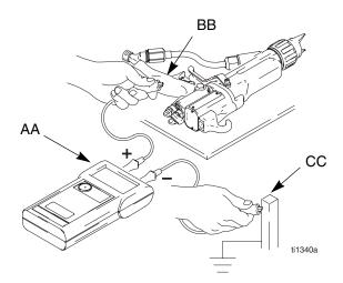
Fig. 3. Check Gun Grounding
