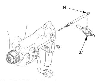
Fig. 14. Fluid Needle Removal
