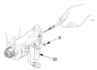
Fig. 15. Fluid Needle Replacement
