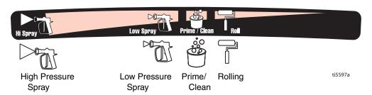
To select function, align arrow on sprayer within range of function symbol on pressure control knob.
