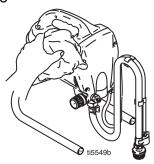
To avoid overheating motor, keep vent holes in shroud clear for air flow.
