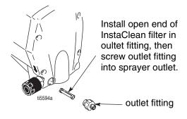
5. Tighten outlet fitting and reconnect hose to sprayer.
