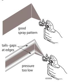
If tails persist when spraying at the highest pressure, a larger tip is needed or the material may need to be thinned.
