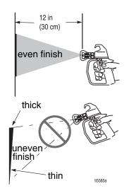
Flex wrist to keep gun pointed straight. Fanning gun to direct spray at angle causes uneven finish.
