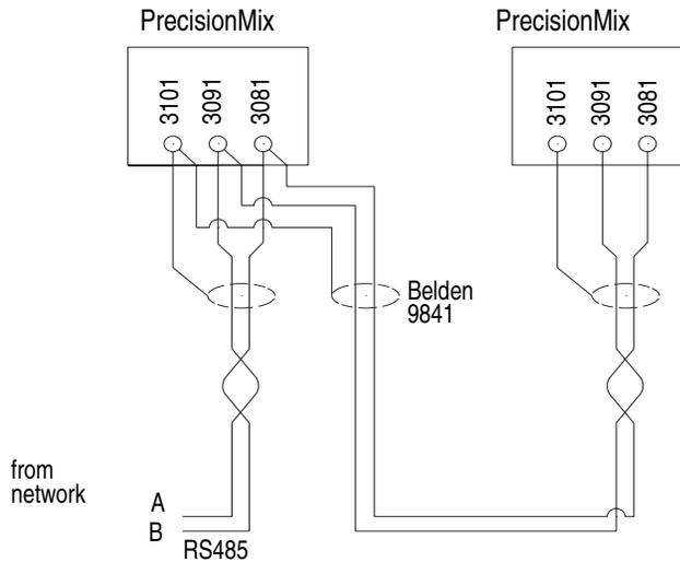
**Figure 12: RS485 connection to PrecisionMix stations**
