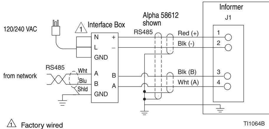
**Figure 7: Informer Station and Interface Box wiring**
