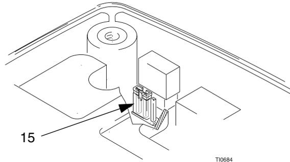
**Figure 9: Jumper position**
