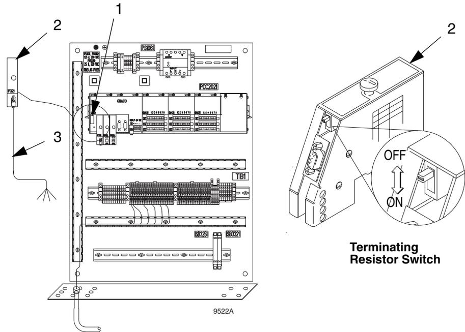
**Figure 10: RS485 Network Module installation**
