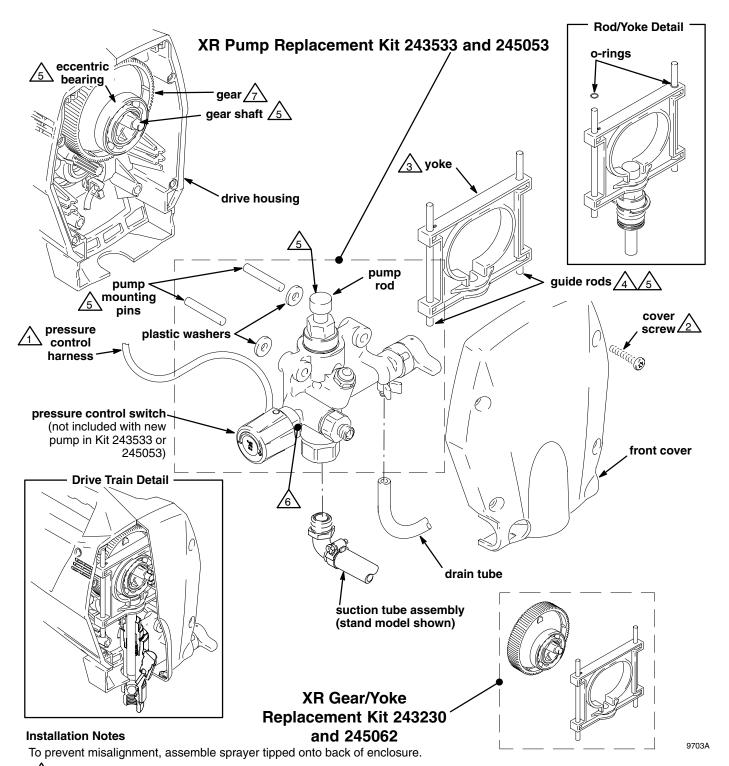
Take care to not pinch harness between pump and any part of drive housing or between front cover and drive housing.
