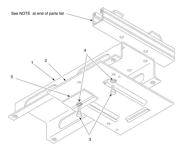
\* Mounts perpendicular or parallel to I-Beam
