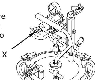
c. Hold down the solvent valve key
