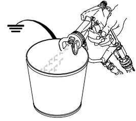
12. Release the component A valve
