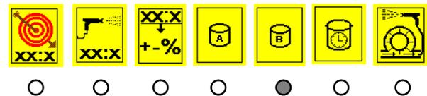
An overdose alarm occurs if the fluid continues to dispense on the one side of the manifold after the valves have opened on the other side of the manifold.
