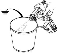
If the fluid section is not clean after completing the purge sequence, repeat the purge by turning the operator switch to standby and back to purge. If the purge time is repeatably too short, change to setup mode and lengthen the purge time.
