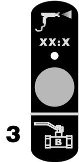
14. Release the component B valve
