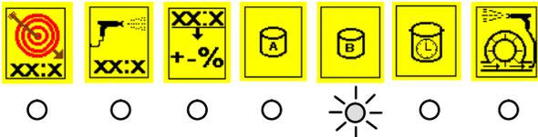
When the air flow switch is activated (gun is triggered), and it takes too long for a dose of A or B to load, the Dose Time A or B Alarm will occur.
