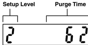
7. Press the arrow keys ( $\Delta\nabla$ ) up or down to change the purge time until the desired value is displayed.
