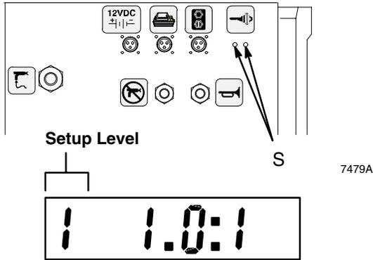
8. Refer to the reference card, and press the return key (↵) on the keypad twice to move to level 3 setup.
